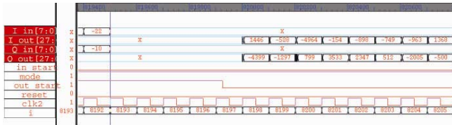
Fig. 8. an illustrative post-layout output waveform of the proposed FFT
