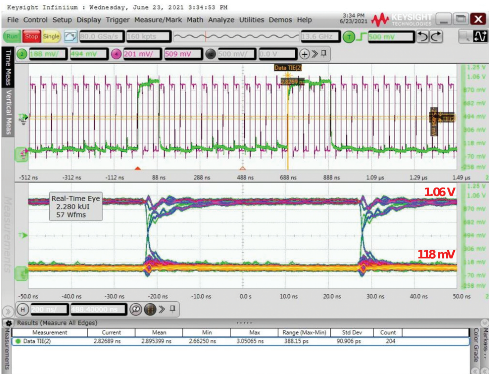
Figure 16. Jitter measurement at a clock frequency of 10 MHz.
