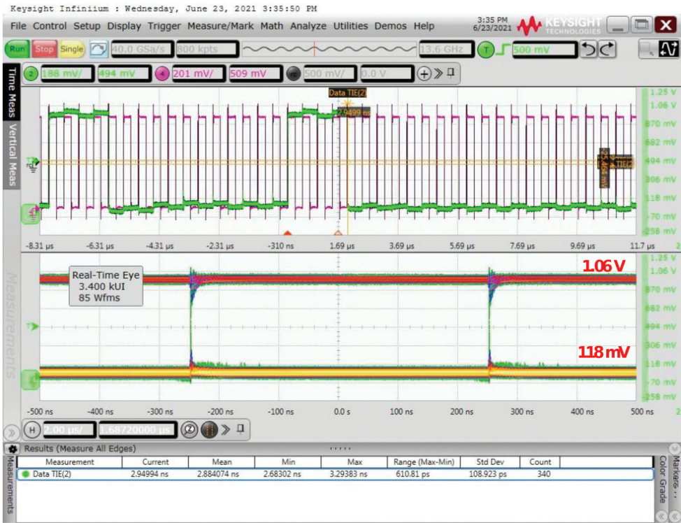
Figure 15. Jitter measurement at a clock frequency of 1 MHz.
